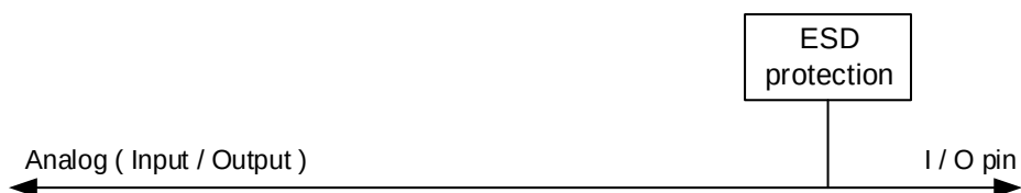
Figure 7-4. Basic structure of Analog configuration
