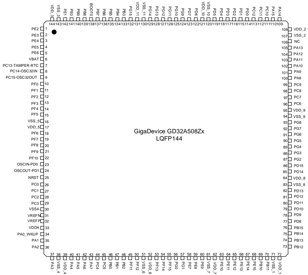
Figure 2-2. GD32A508Zx LQFP144 pinouts
